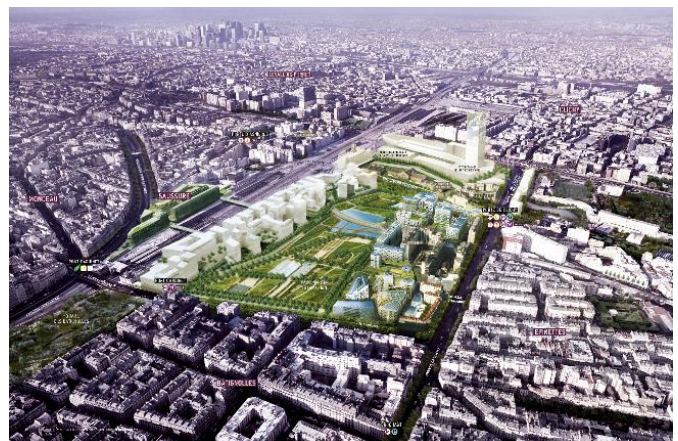
FIGURE 4.19 Perimeter blocks in central Paris, France. Perimeter block development has a number of advantageous characteristics/features: explicit public and private sides, the capacity to accommodate different densities of development; and a public façade that both physically defines and 'socially' addresses an urban space
