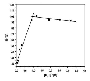
**Fig. 4** Determination of the stoichiometry of the extracted copper(II)-H<sub>2</sub>SALEN complex by the mole ratio method.  $[Cu^{2+}] = 1.57 \times 10^{-3} \text{ mol/L}; \text{ pH} = 8; \text{ [Na<sub>2</sub>SO<sub>4</sub>]} = 0.5 \text{ mol/L}; T = 60 °C \rightleftharpoons$
