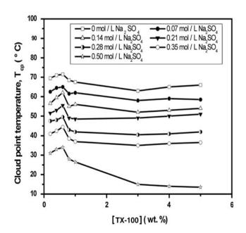
Fig. 3 Phase diagram of TOP9.5EO-water-Na<sub>2</sub>SO<sub>4</sub> ternary systems
