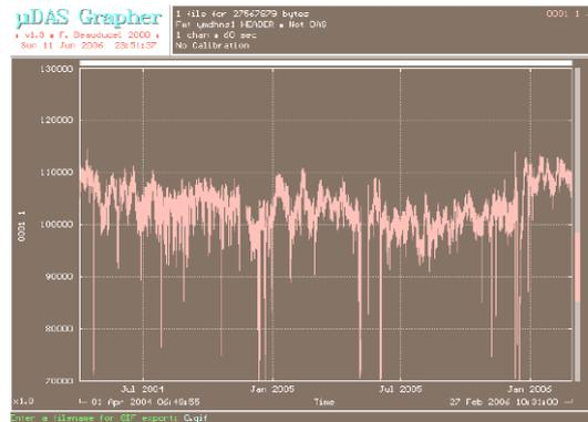
Fig. 2 Raw Recordings of the electronic tide gauge of Algiers, Period: March 29, 2004 to February 27, 2006.
