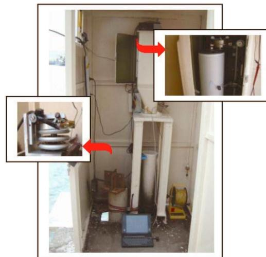
**Fig. 1** Tidal gauge site of Algiers sheltering the two tide gauges electronic (in the left) and analogical (in the right).
