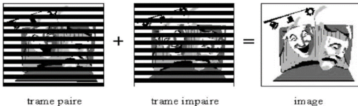
Figure II.1. Principe de transmission analogique. [17]
