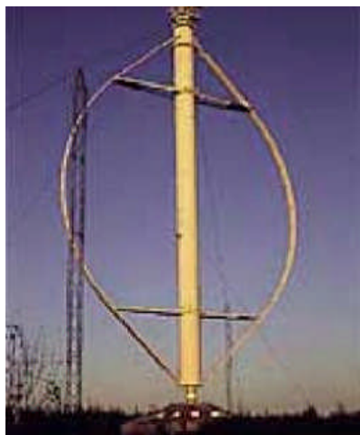
Figure I.2 : Structure de Darrieus
